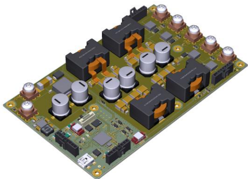
CON locking Connector equipped version (Best suited for series production)
