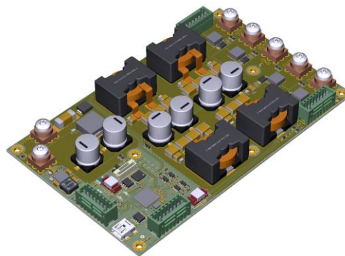
TB Terminal Block equipped version (Best suited for prototyping, commissioning and small series. Attention: Counter parts for Terminal Blocks will not be shipped with the device!)
